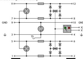
Complete module indirect grounding, with remote signalling
