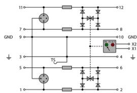
Complete module direct grounding, with remote signalling
