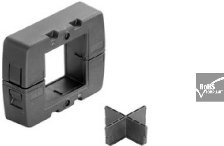
The frame, fabricated from a single piece, is quick and easy to assemble and consists of dimensionally stable, fibre-glass reinforced plastic. The captive foamed seal guarantees effective IP66 sealing in accordance with DIN EN 60529, even on painted and rough surfaces.
