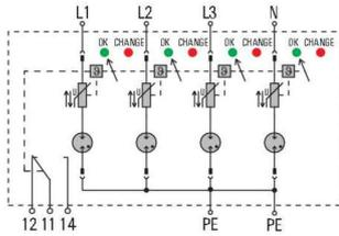
Schematic circuit diagram
