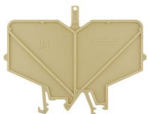
Support brackets can be arranged at the end or in the course of a terminal strip. They can be clipped on TS 32 or TS 35 mounting rails and serve as supports for the respective cover profiles.
