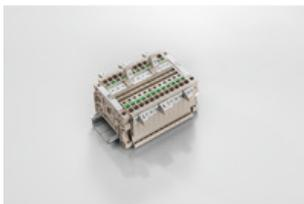
The marker holder offer the possibility of additional mounting of standard markers with a pitch of 5 or 5.1 mm. The angled holders can be optionally snapped together and could be mounted in all standard marking channels of the Klippon<sup>®</sup> Connect modular terminal blocks. Fitting marker types could be found under the respective accessories of the designation marking holder.
