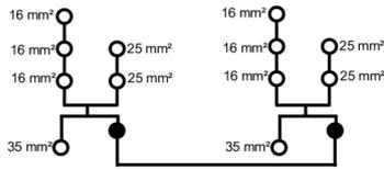
Conductor connection data according to IEC 60947-7-1 (Cu)
