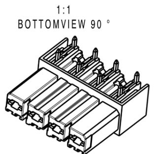
For the mounting of PCBs, it should be noted that the rated data given in the catalogue relates only to the connection elements. The necessary creepage and clearance paths must be observed in connection with the respective applicant in accordance to VDE 0110. The current-carrying capacity and pitch tolerance is to be determined according to DIN IEC 326 part 3 very fine.
