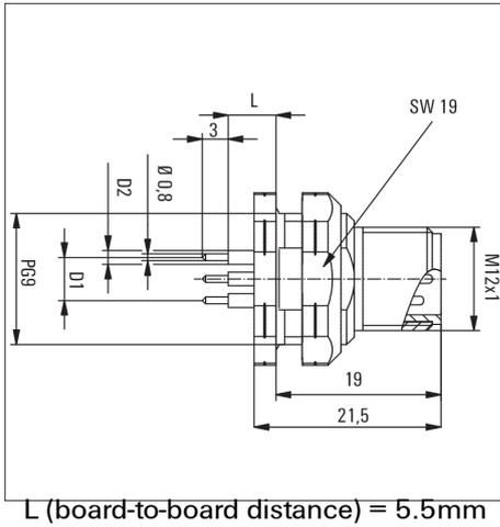
**Front panel section** D1 = 5,0 mm
