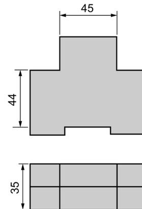
Suitable RCBO for the RCBO cut-out has the dimensions in the drawing (acc. to DIN 43880). Every RCBO with this dimension will fit.
