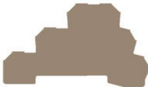
To ensure the finger safety and the compliance to the required clearance and creepage distances, an end plate has to be placed at the end of a plug.
