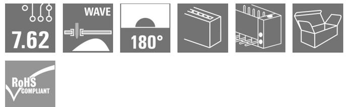
180° male header with middle flange with a 7.62 pitch. Meets the requirements of IEC 61800-5-1 and enables UL approval as per UL840 600 V.
