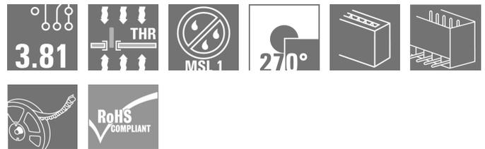
The SC-SMT pin header in 270°-outlet direction: the 270° angle exists between the plugging direction and the solder pin. The plugging direction is then parallel to the PCB. Sockets blocks, however, have an overhead plugging angle.
