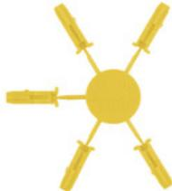
Through the use of coding pins, individual coding options ensure trouble-free plug-in connection.
