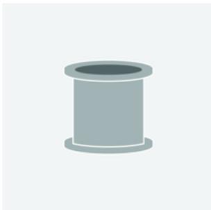
Gauge rings are used to protect against the using of incorrectly selected fuse sizes. They are simply inserted into the respective fuse base and prevent the using of bigger fuses.
