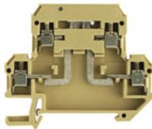
In some applications it makes sense to add a test point or a disconnect element to the feed through terminal for testing and safety purposes. With test disconnect terminals you measure electric circuits in the absence of voltage. While the disconnecting points clearance and creepage distance is not assessed in dimensional terms, the specified rated impulse voltage strength must be proven.
