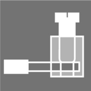
M12 plug-in connector in IP 67 available with screw or tension clamp connection
